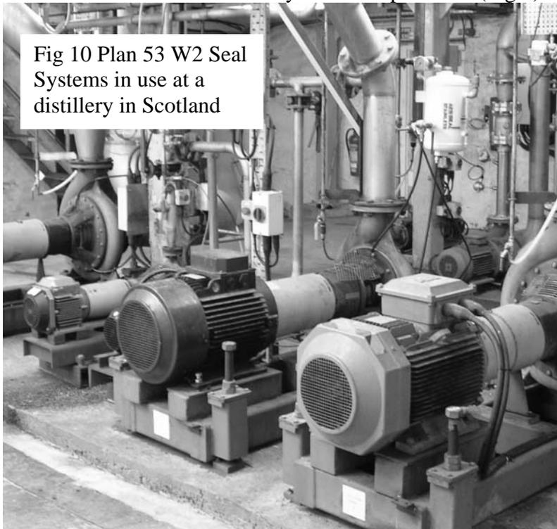
Fig 10 Plan 53 W2 Seal Systems in use at a distillery in Scotland
