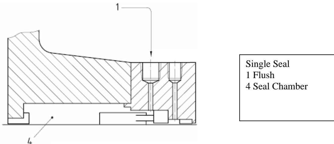
Fig 3a Typical single seal Piping Plan
