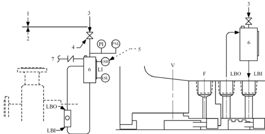
Pressurised external barrier fluid reservoir supplying clean fluid to the seal chamber. Circulation is by an internal pumping ring. Reservoir pressure is greater than the process pressure being sealed.
