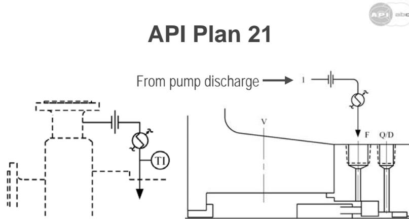
Recirculation from pump discharge through a flow control orifice and cooler, then into to the seal chamber.
